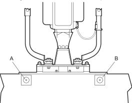
2. Set the operating handles in working position by using the lock levers.
